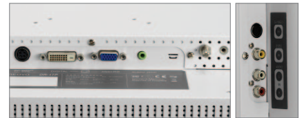
Analogue, DVI, S-Video and CVBS inputs for video device or PC data feeds
